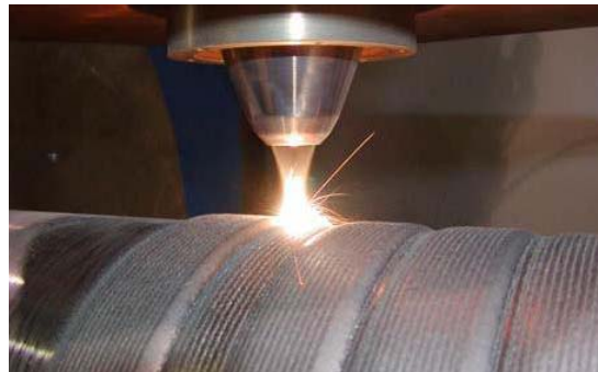
Figure 3: Laser cladding process set up [5].
